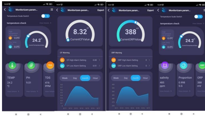
Fig. 5. Monitoring water quality parameters in the aquaculture system on a smartphone.
