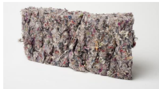
Fig. 4. Recycled cashmere insulation
