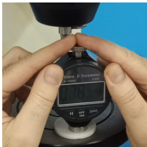
Fig. 6. The device for measuring the hardness of ABS parts
