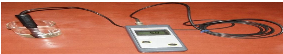
Fig. 3 Determination of oxygen content in small aliquot of aerated water using HANNA instrument with polarography sensor [1]
