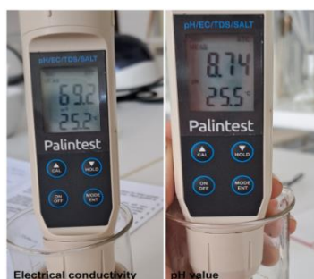
Fig. 7. Reading of soil conductivity and pH value
