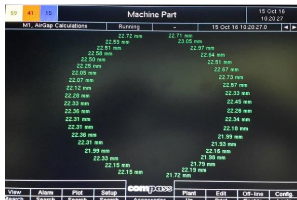
Fig. 5. Analysis of the air gap on Hydro power unit No. 1
