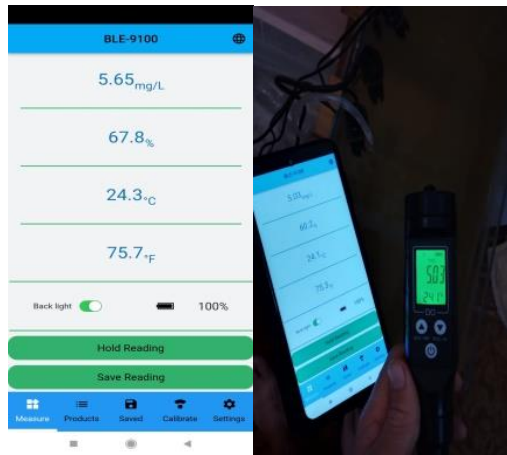
Fig. 6. Monitoring the dissolved oxygen level in the aquaculture system on a smartphone.
