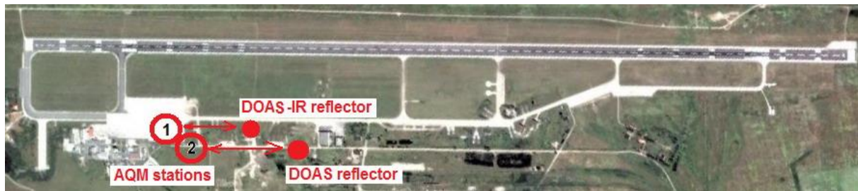
Fig. 4. Timisoara international airport lane and DOAS (1 and 2) set-up.
